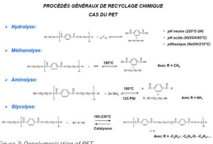
*Figure 3: Depolymerisation of PET Source: Enscm: www.enscm.fr/en/*
