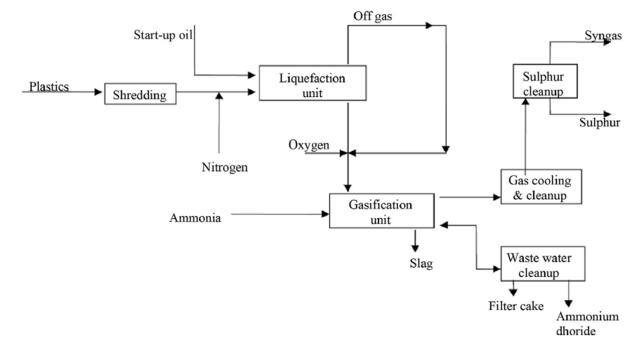
*Figure 4: The Texaco gasification process schematic diagram Source: Brems et al., 2015 Gasification Of Plastic Waste AsWaste- To- Energy Or Waste- To- Syngas Recovery Route, Solid Waste as a Renewable Resource. Apple Academic Press, pp. 241–263.*
