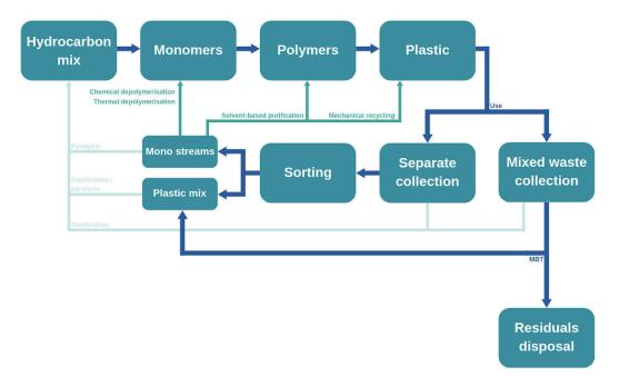
*Figure 1: Diagram of different chemical recycling processes Source: Zero Waste Europe: <u>www.zerowasteeurope.eu</u>*
