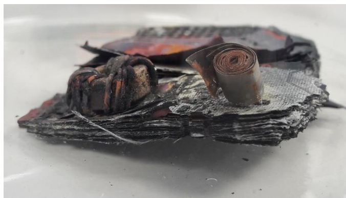
Figure 33. PCB glass fibre layers
