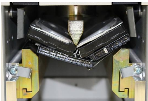
Figure 14. Crushing of drives (source: www.veritysystems.com )
