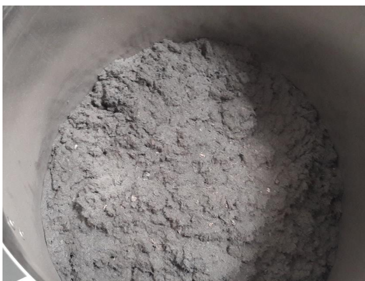
Figure 31. PCB after cutting mill
