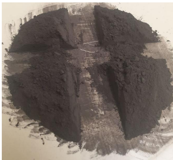
Figure 32. Sampling process of the black powder after vibrating disc mill.
