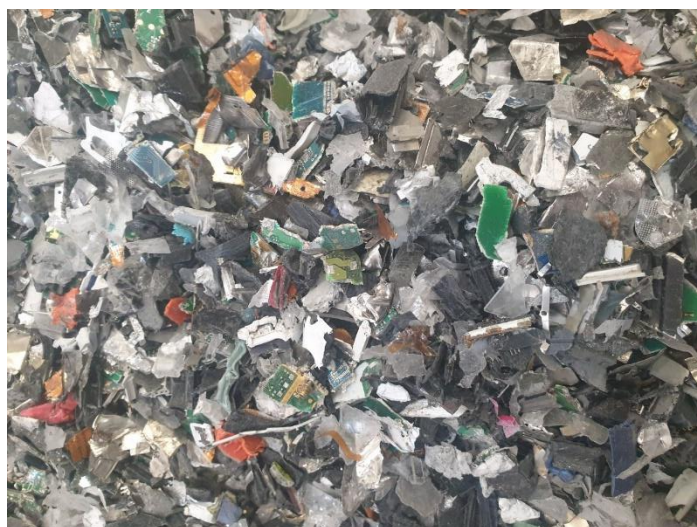
Figure 13. Shredded drives (source: CEDaCI dismantling and characterisation)
