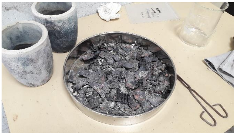
Figure 30. PCB after pyrolysis
