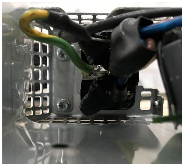
Figure 25. PSU connection (SV.1.2.9.1.2). Difficult access to screws.
