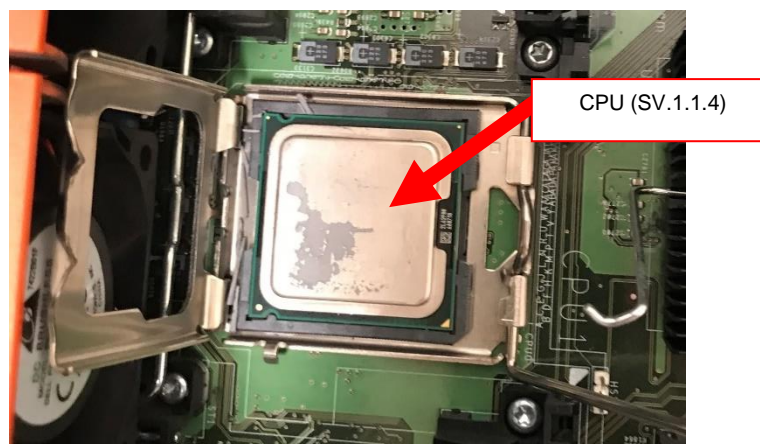
Figure 19. CPU present under heat sinks (SV.1.1.4)
