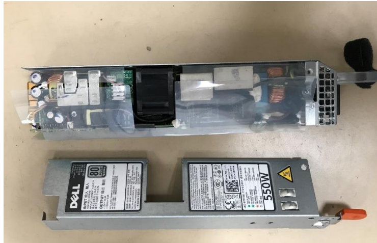
Figure 24. Open PSU1201D (SV.1.2.9.1)
