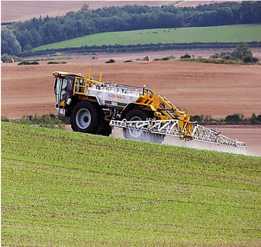
Fig. 77. A Lite-Trac four wheeled self-propelled crop sprayer, putting pesticide on a field, with many thanks to Wikipedia and the Author.
