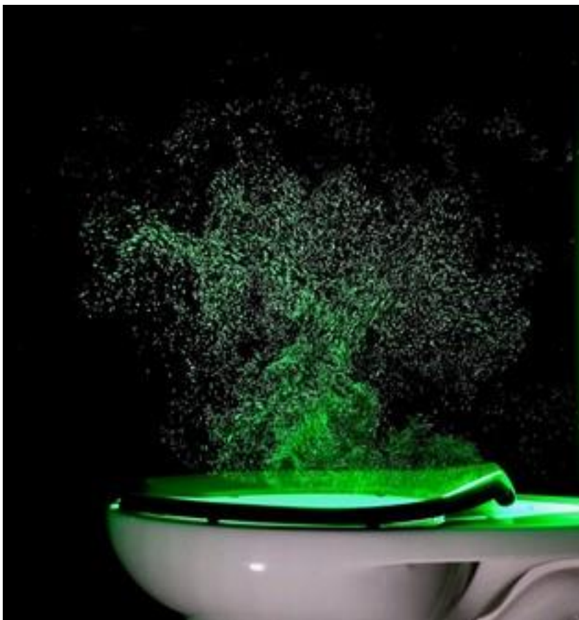
Fig. 26. Aerosol plumes from traditional flush FaF toilets can rise up to 5 feet above the bowl, and remain suspended in air, exposing people to disease vectors, with many thanks to the Authors (Crimaldi, 2022).
