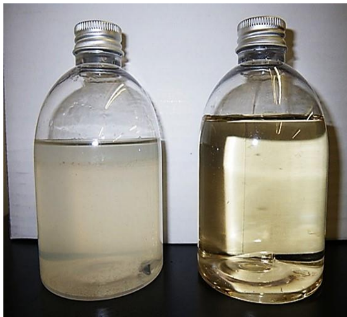
Fig. 57. Left: Greywater sample from an office building. Right: Same grey water after treatment in membrane bioreactor, with thanks to the SuSanA
