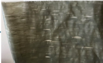
Contaminated film with defects → SOA recycling not applicable
