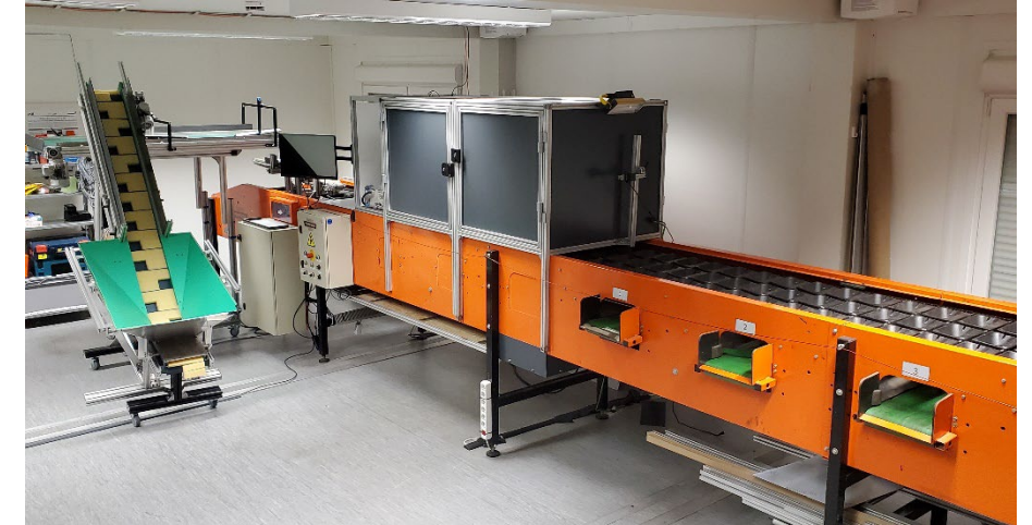
Sort4Circle demo line: Singulation, two detection chambers, tray sorter
