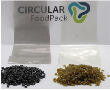
Recyclate and 100% PCR film without and with additional purification
