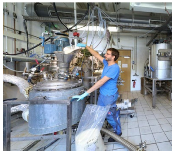
Small-Technical Scale 5-10 kg per day using stainless steel equipment (100-250 L)
