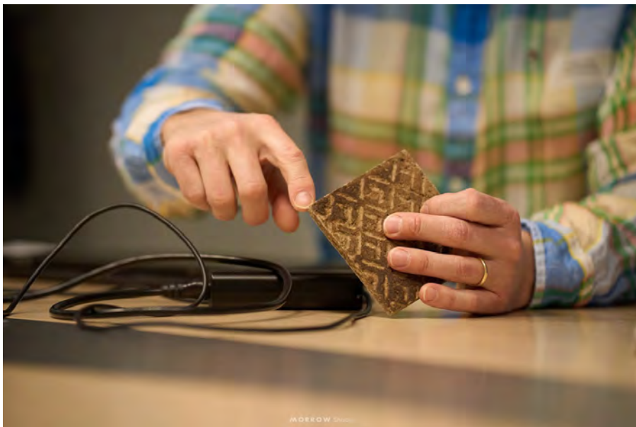
Picture 3. Prototype of hemp-based construction board developed in Central Finland (Photographer: Morrow Shoots)
