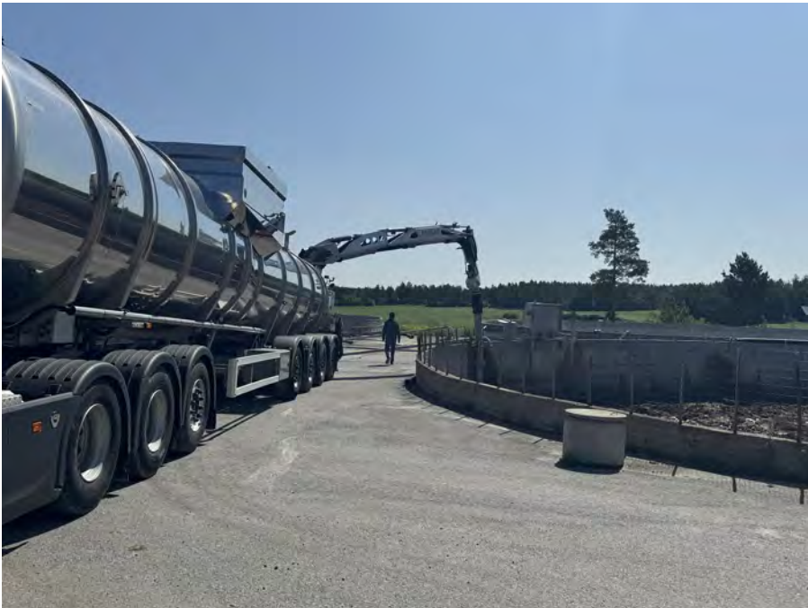
Picture 1. A slurry tanker on the left pumping digestate from a storage tank on the right during nutrient recycling operations (Photographer: Tero Liukas Oy)
