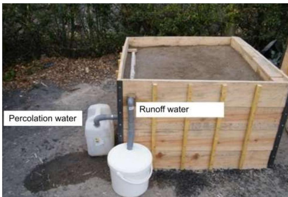
**Figure 18. Experimental board implemented for an application in road sub-layer**
