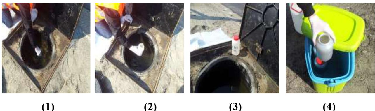
Figure 26. Collection of percolation water at the experimental site (Achour, 2013). (1) and (2) Sample Collection, (3) and (4) Packaging.
