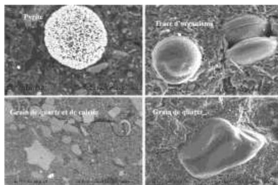
**Figure 12. Scanning electron microscopy (SEM) photomicrographs of a marine sediment** (trace d'organisme = organism image, Grain de quartz = quartz grain)
