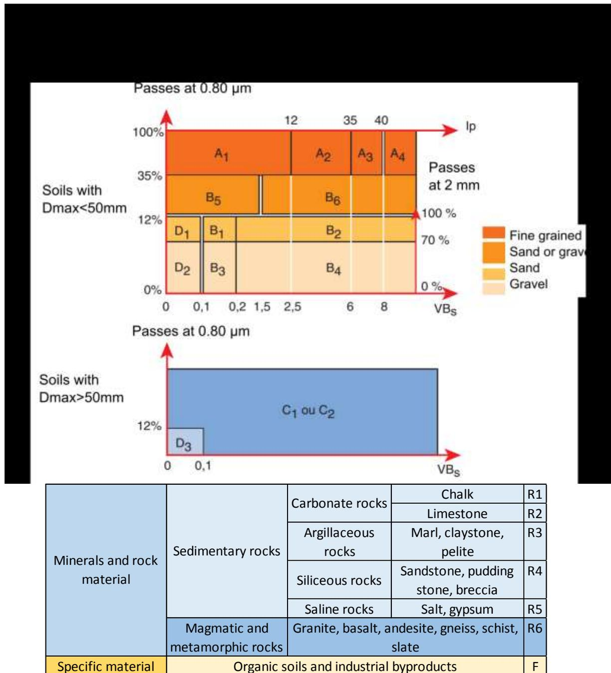
Figure 11. Synoptic classification of materials according to their nature, according to standard NF P 11-300 (CIMBETON, 2009)
