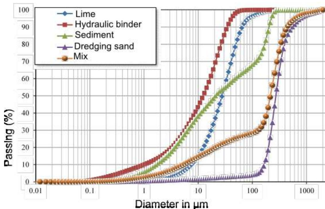
Figure 13. Particle size distribution of constituents of a road material
