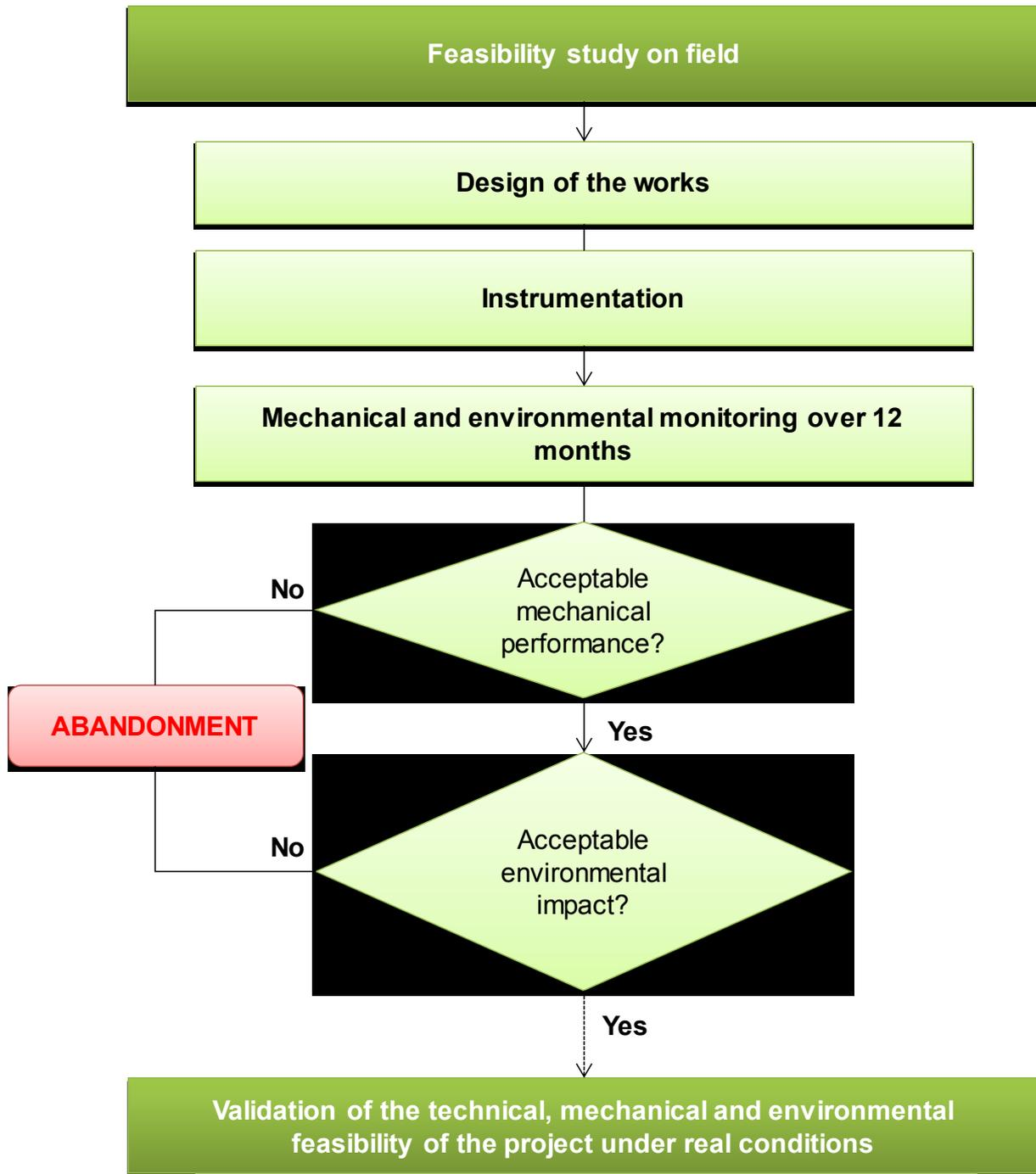
Figure 32: PHASE 3B: Pilot field test
