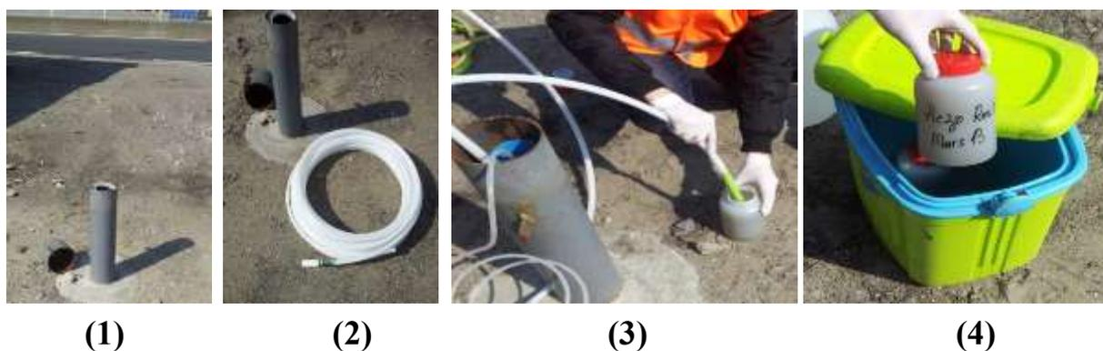
**Figure 27. Water sampling at the piezometer. (1) Piezometer, (2) Valve pump, (3) Sampling device, (4) Sample conditioning**
