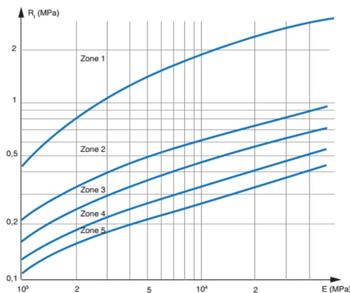
Figure 15. Classification chart for road structure materials with hydraulic binders (SETRA-LCPC, 2000)
