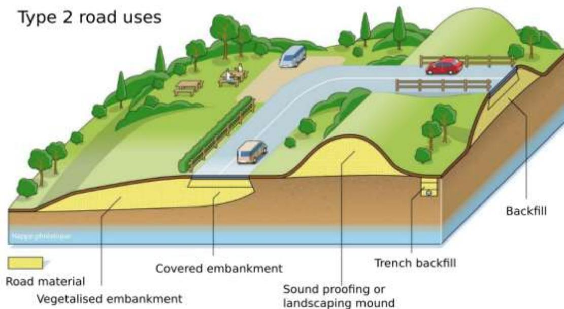
Figure 4. Illustration of 'type 1' and 'type 2' road uses (adapted from SETRA, 2011)
