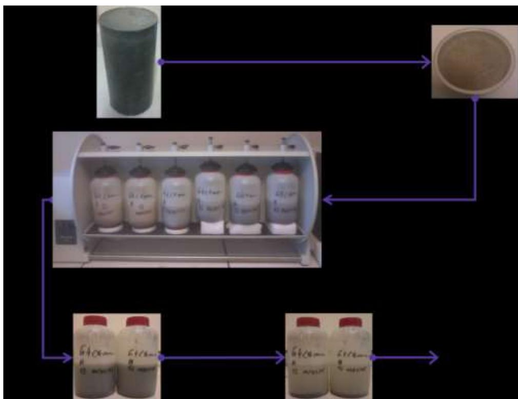
**Figure 16. Main steps of a leaching test carried out according to standard NF EN 12457-2**
