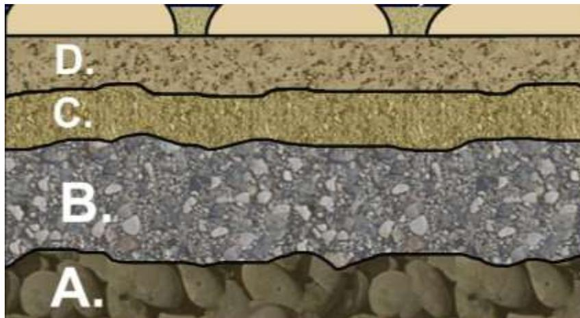
A.) Subgrade B.) Subbase C.) Base course D.) Paver base (may be paved or covered by asphalt)
