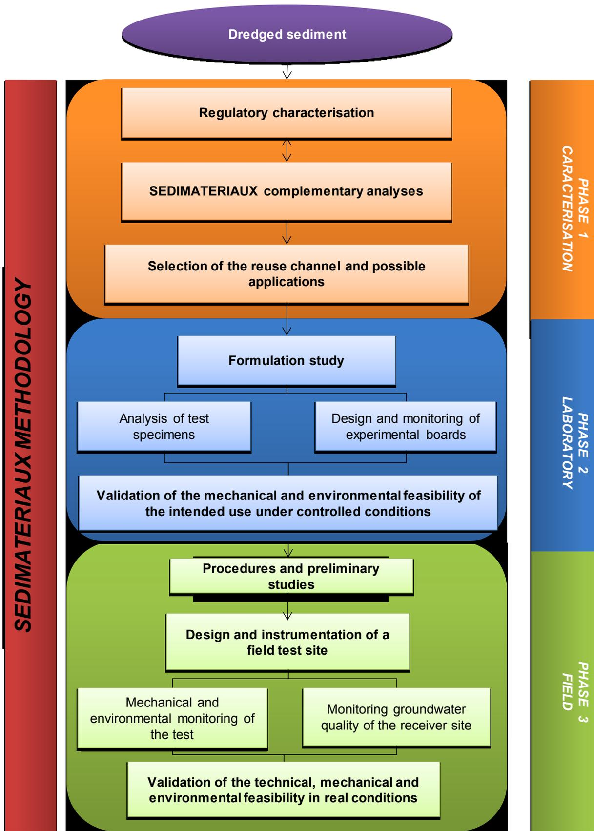
Figure 7. Description of the methodology developed as part of the SEDIMATERIAUX approach
