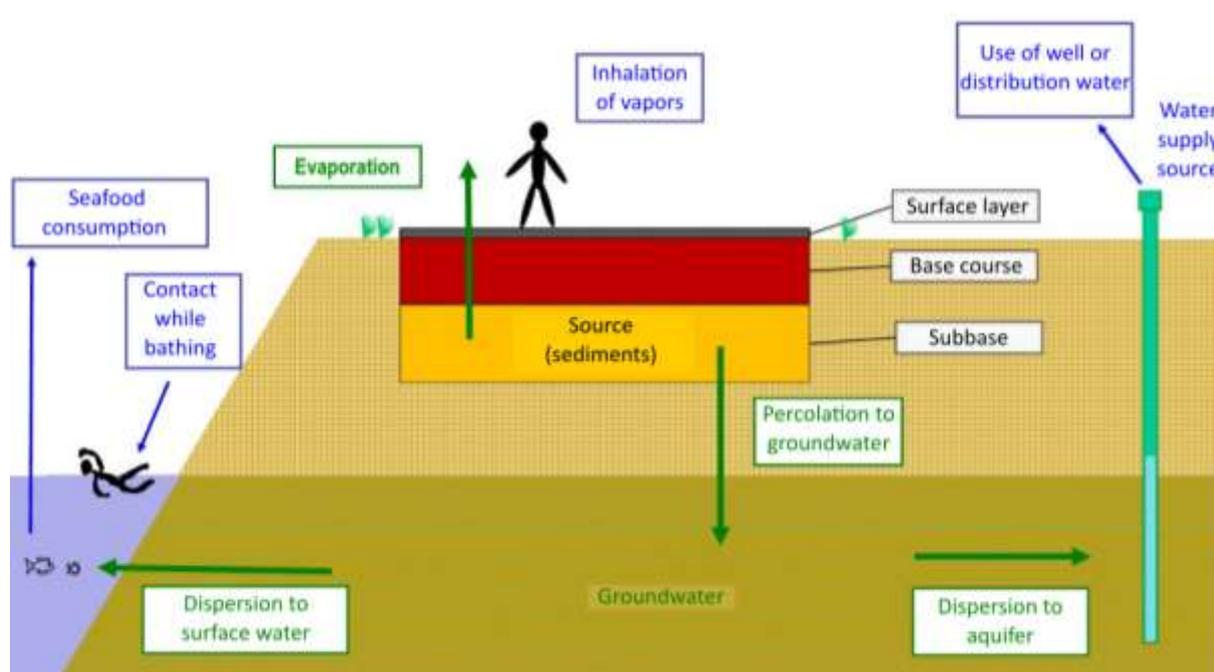
Figure 23. Conceptual diagram of the environmental and health risk assessment of a sediment-based road structure (From: IDRA Environnement)
