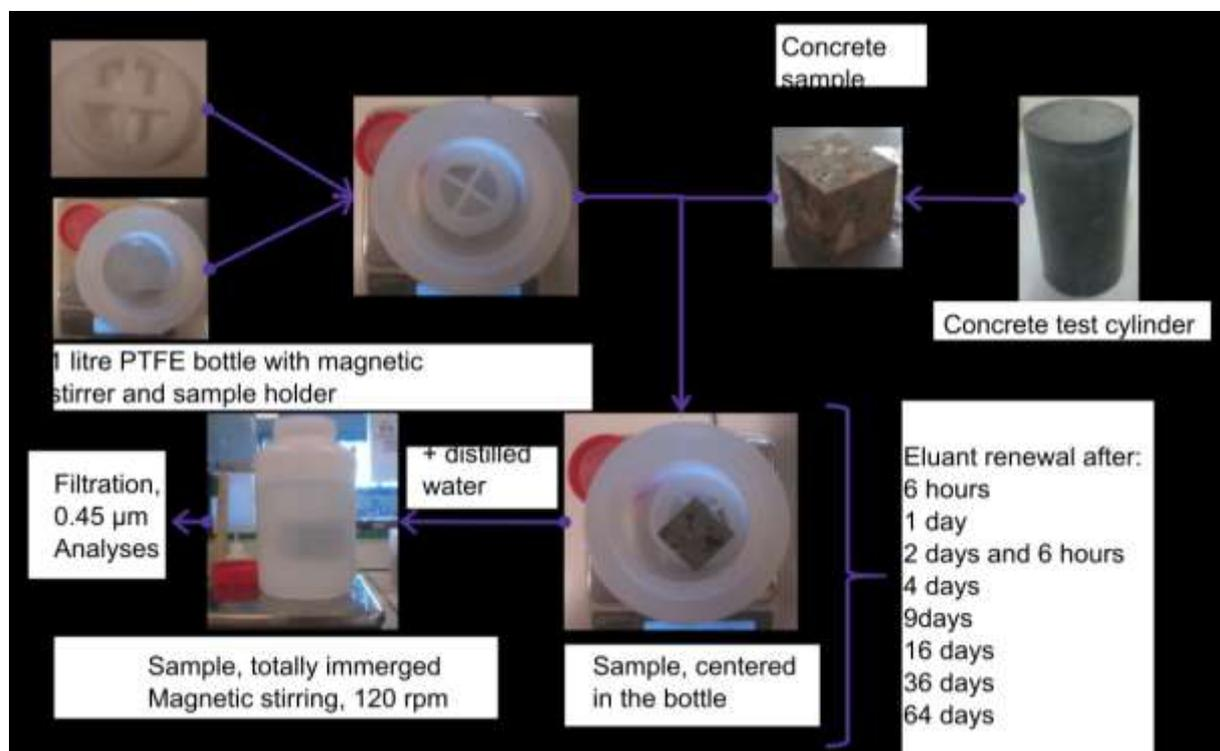
Figure 17. Experimental set-up for leaching on monolith with leaching agent renewal
