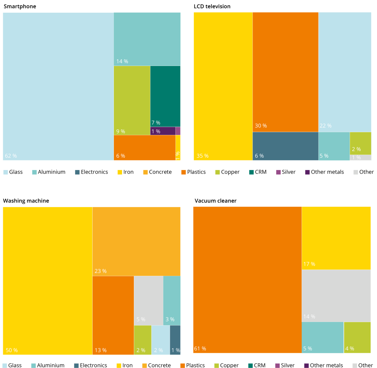
Figure 4. Average content of a smartphone, LCD television, washing machine and vacuum cleaner.
