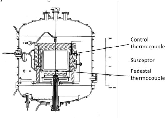
**Figure 5:** Schematic of the Crystalox DS-250 furnace at SINTEF.
