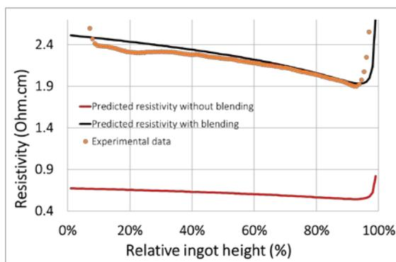
**Figure 17 :** Resistivity profile along relative ingot height (reporting data of middle of one lateral side). Comparison with predicted resistivity without and with blending with EG-Si.
