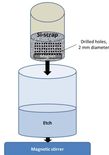
**Figure 3:** Principle sketch of the setup used for the small scale experiments at SINTEF (not to scale).
