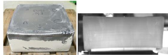
**Figure 13:** Picture of the ingot casting by directional crystallization done at CEA (at left) and IR transmission imaging.
