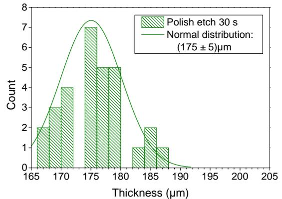
**Figure 11:** Thickness distribution histogram of 30 samples from the SOLITEK material after small scale etching in 30 seconds. Thickness before etching is given in Figure 9.
