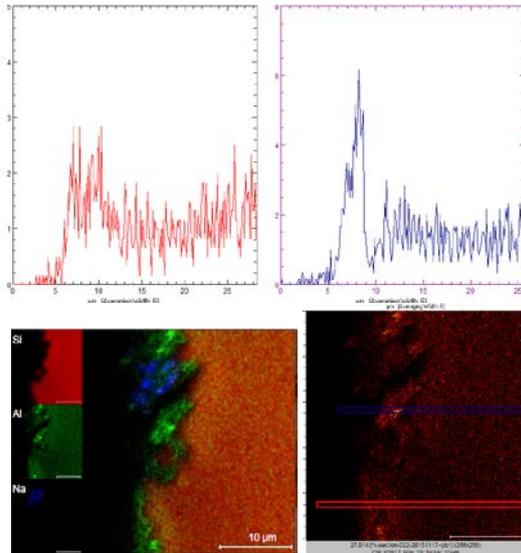
**Figure 2:** ToF-SIMS analysis of the back side of Si solar cell structure after removal of front and back side contacts. The upper graphs are two line scans for aluminium along the lines in lower right picture.
