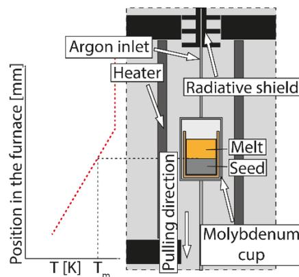
**Figure 12:** Bridgman tube furnace at NTNU in Trondheim, Norway [8].
