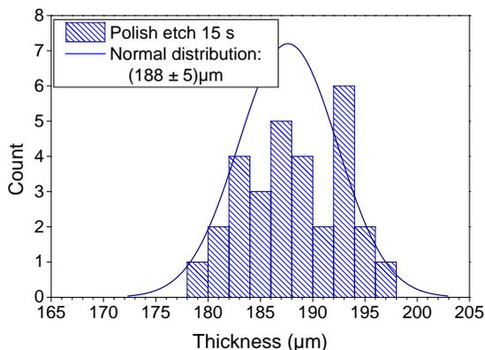
**Figure 10:** Thickness distribution histogram of 30 samples from the SOLITEK material after small scale etching in 15 seconds. Thickness before etching is given in Figure 9.
