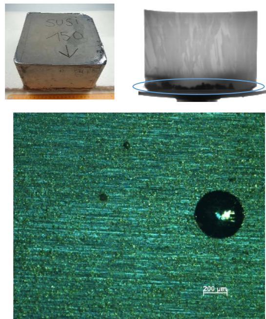
**Figure 16:** Silicon ingot picture (at left), IR transmission imaging of the ingot (at right) and optical microscopy imaging (c) of the dark bottom part (Fig 15.b) revealing cavity like defects.
