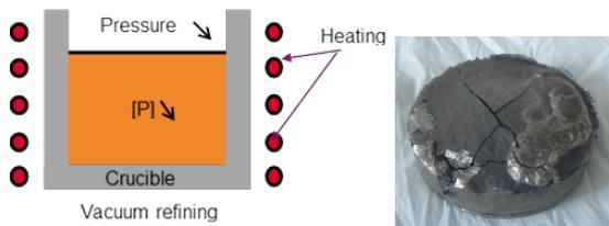
**Figure 15:** Schematic vacuum induction melting process (at left) and picture of the purified Si-ingot (2.46kg) (at right).
