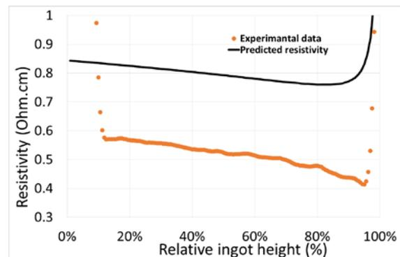
**Figure 14:** Resistivity profile of G2 ingot from etched silicon along relative ingot height.
