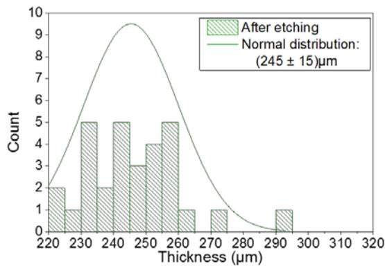
**Figure 8:** Thickness distribution histogram of 30 samples from the LOSER material after small scale etching at SINTEF. Thickness before etching is given in Figure 6.
