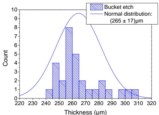
**Figure 7:** Thickness distribution histogram of 30 samples from the LOSER material after large scale etching at SINTEF.
