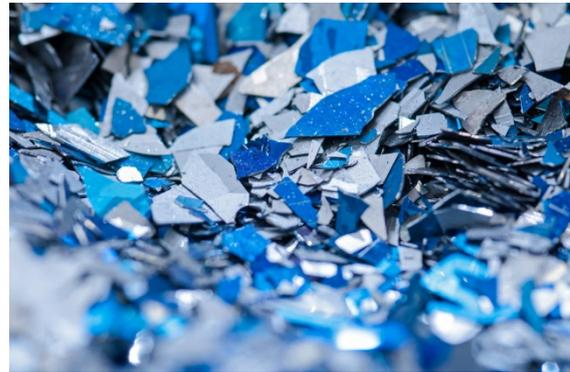
**Figure 1:** Broken solar cell pieces (Si-shards) delivered from LOSER Chemie. The front finger and Al back contacts have been removed. The size of pieces are about 2 - 20 mm. (courtesy LOSER Chemie GmbH).
