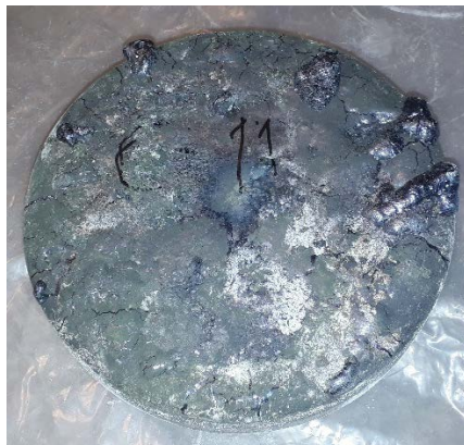
Figure 6: Photo of the ingot with 100 % refined material.
