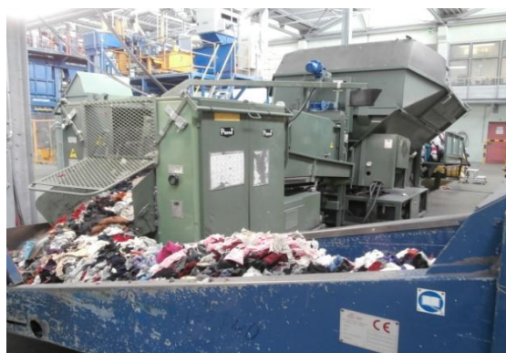
Figure 9: Textile recycling - cutting of textile waste vs Textile recycling - resulting fibres [39]
