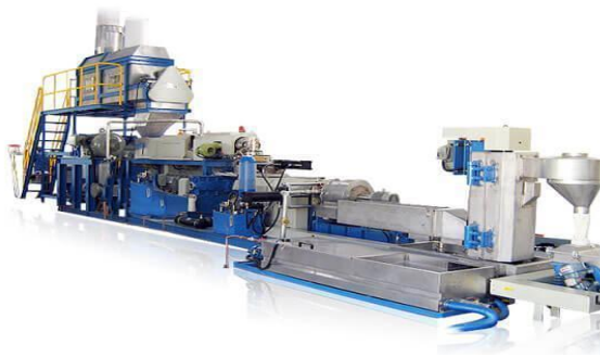
Figure 10: The extrusion-pelletizing line [40]
